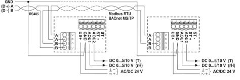
Wiring RS485 (Modbus RTU & BACnet MS/ TP)
